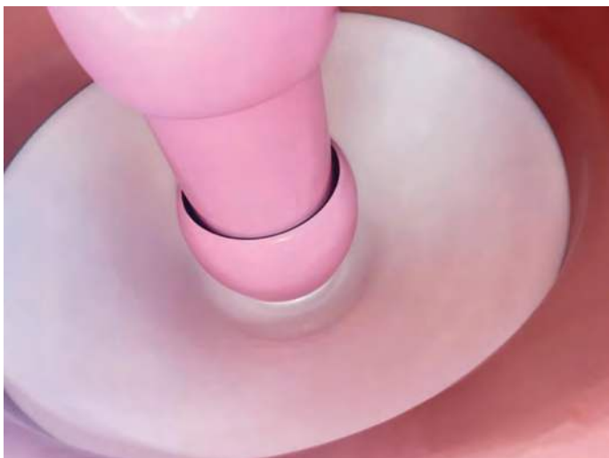
Figure 3. Schematic diagram of the inner metal guide rod–basin insulator.
