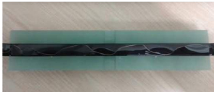
Figure 17. Catastrophic failure of polyetherimides (PEI)–polyamide imides (PAI)–coated wire sample specimen aged at 200°C [9].
