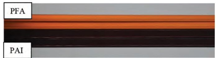
Figure 9. Comparison of perfluoroalkoxy (PFA) and polyamide imides (PAI) wire before tests.
