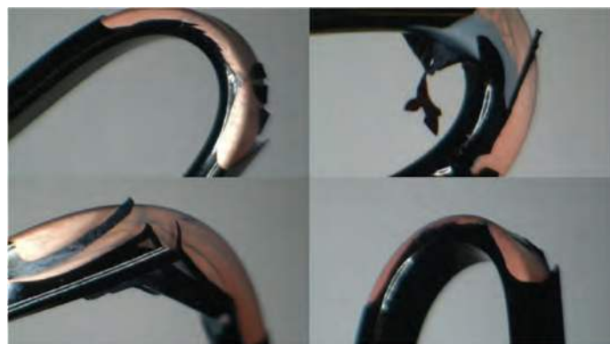
Figure 15. Polyamide imides (PAI) wire after 2,000 hours at 150°C in oil tester.
