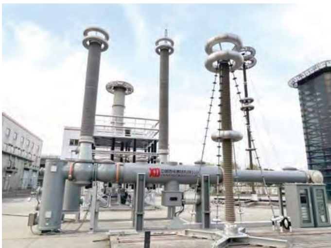
Figure 1. Schematic diagram of the long-term electrification test for the \pm 550 -kV DC gas-insulated switchgear.
