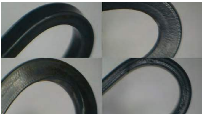
Figure 16. Perfluoroalkoxy (PFA) wire after 2,000 hours at 150°C in oil tester.
