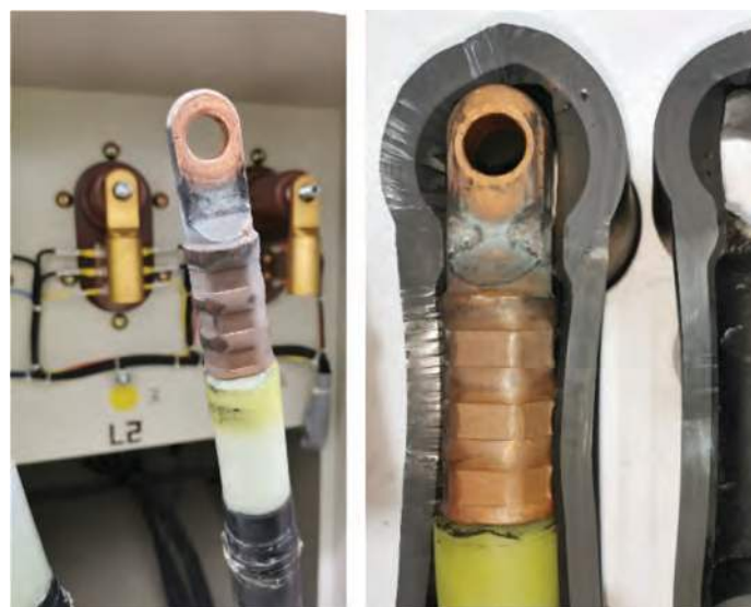
Figure 12. Discharge marks at the terminations.
