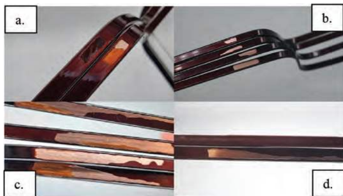
Figure 12. Defects of polyamide imides (PAI) wire after thermal aging with additional stress: (a) after 24 hours at 180°C; (b) after 24 hours at 200°C; (c) after 24 hours at 240°C; and (d) wire comparison after 24 hours at 240°C. Perfluoroalkoxy (PFA) wire at the top, and PAI wire at the bottom.
