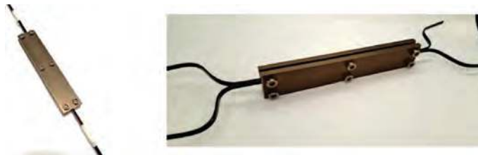
Figure 3. (left) View of sample and metal plates; (right) view of the sample with bent wire ends, ready for testing.
