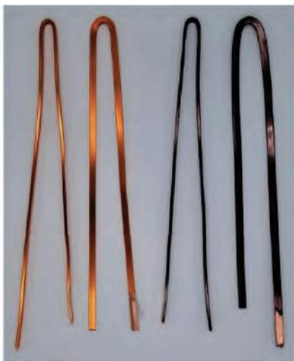
Figure 4. The appearance of samples for the breakdown voltage study with different types of bending with mandrel—flat and edge.
